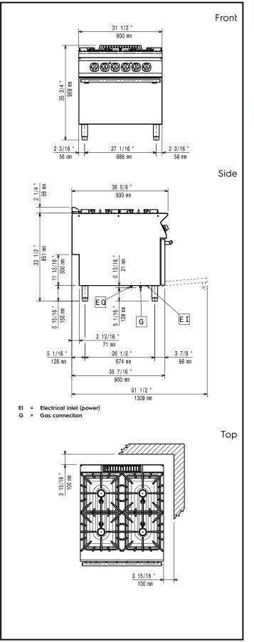
Modular Cooking Range Line 900XP 4-Burner Gas Range on Electric Oven
